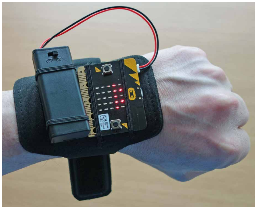
Figure 1: BBC micro:bit and AAA battery pack on a home-made wrist holder.
