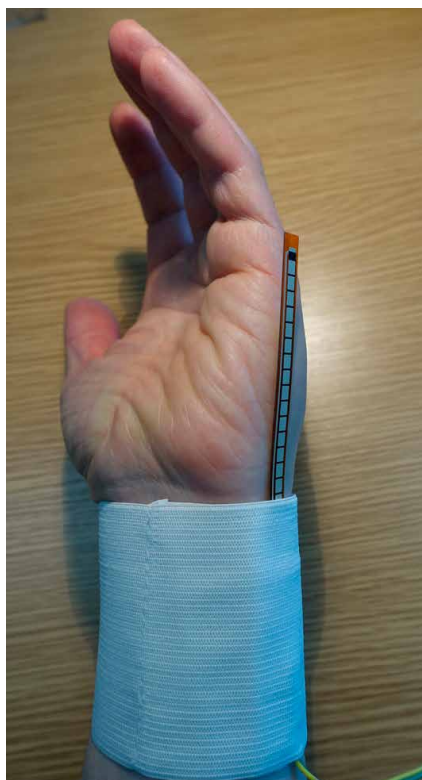
Figure 2: Flex sensor held in position to detect a sideways hand motion.
