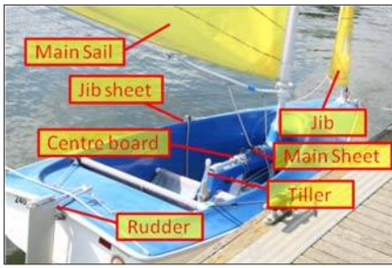
Figure 1 Parts of the boat
